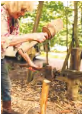
Removing timber to just above finished size
